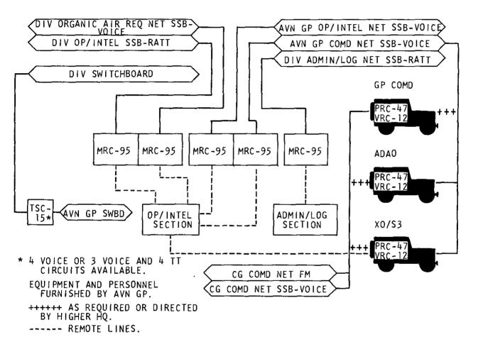
Figure 15-2. Aviation group type radio net.
