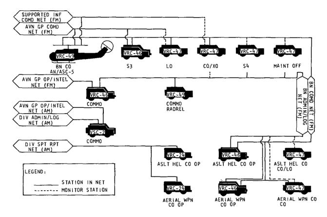
Figure 17-2. Type assault helicopter battalion radio net.
